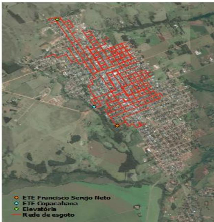
FIGURA 6: COBERTURA DA REDE COLETORA DE ESGOTO DE AMAMBAI.
